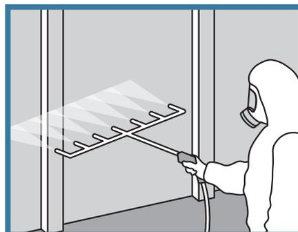
a pistol grip. If no water supply is readily available, a portable pressurised vessel (for example, a pump-up garden sprayer) may be used.
