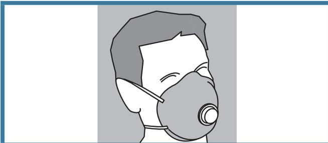
FIGURE 5: Disposable, half-face particulate respirator.
