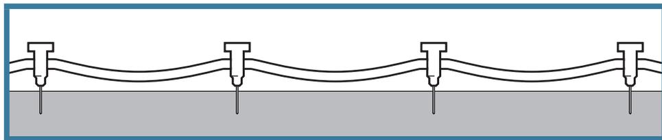
The asbestos is soaked by the introduction of water or other wetting agents through an appropriate applicator that consists of an injection head with numerous side holes or outlets through which the water or wetting agent is fed to the asbestos.
