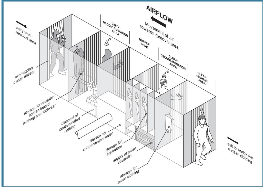
The decontamination unit should be immediately adjacent to and directly connected with the enclosed removal work area. It should be located as far away as practicable from workplace facilities such as and lunch rooms
