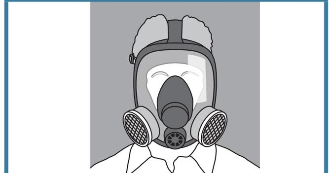
FIGURE 8: Full-face, particulate filter (cartridge) respirator.
