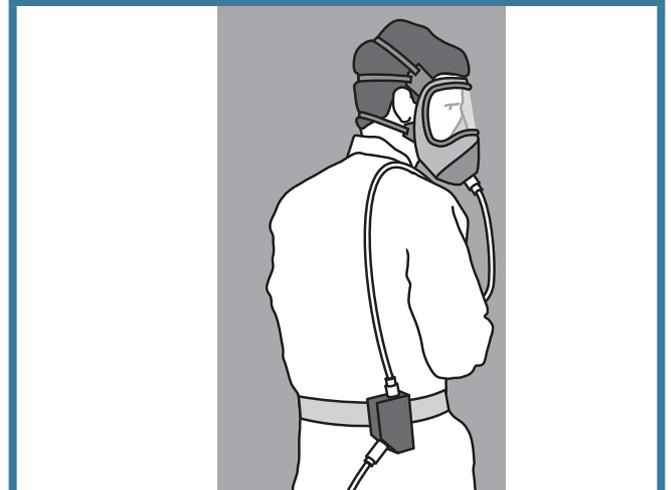
FIGURE 10: Full-face, positive pressure demand air-line respirator.
