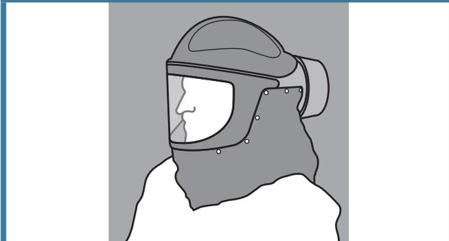
FIGURE 7: Powered, air-purifying, ventilated respirator.
